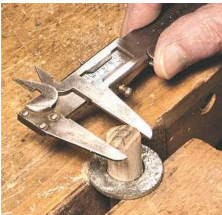
▲ Pic. 7 You need to check the filing with a Vernier calliper gauge
